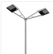
14068794 Twin WIN+2 aluminium pole top fitting and steel outreach arm for Ø76mm poles, installed at 90°. Painted aluminium grey
